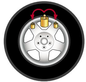
“**Hidden Weight**” program (in Alu P) which subdivides the adhesive weight for the outside into two equivalent weights positioned behind the spokes of the rim
